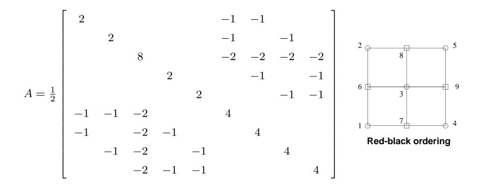
The idea of this ordering is to get a stiffness matrix in a block form where the diagonal blocks are diagonal matrices. This allows for efficient 1D parallel decomposition.
