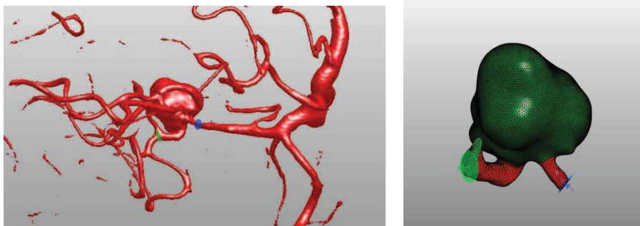
Figure 1: Blood vessels geometry (left), mesh generation at the region of interest (right).
