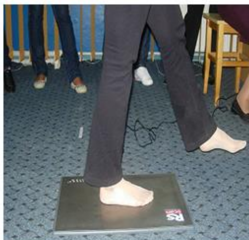
Fig. . The use of the Footscan plate: a) outside of walking route, b) included in a walking route of 6 m.
