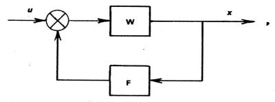
where W is a linear stationary (time-invariance) element, F is a nonlinear element and u is a control signal.
