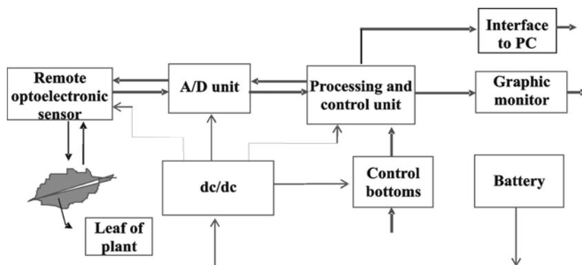
Fig. 2. Functional diagram of portable device "Floratest"
