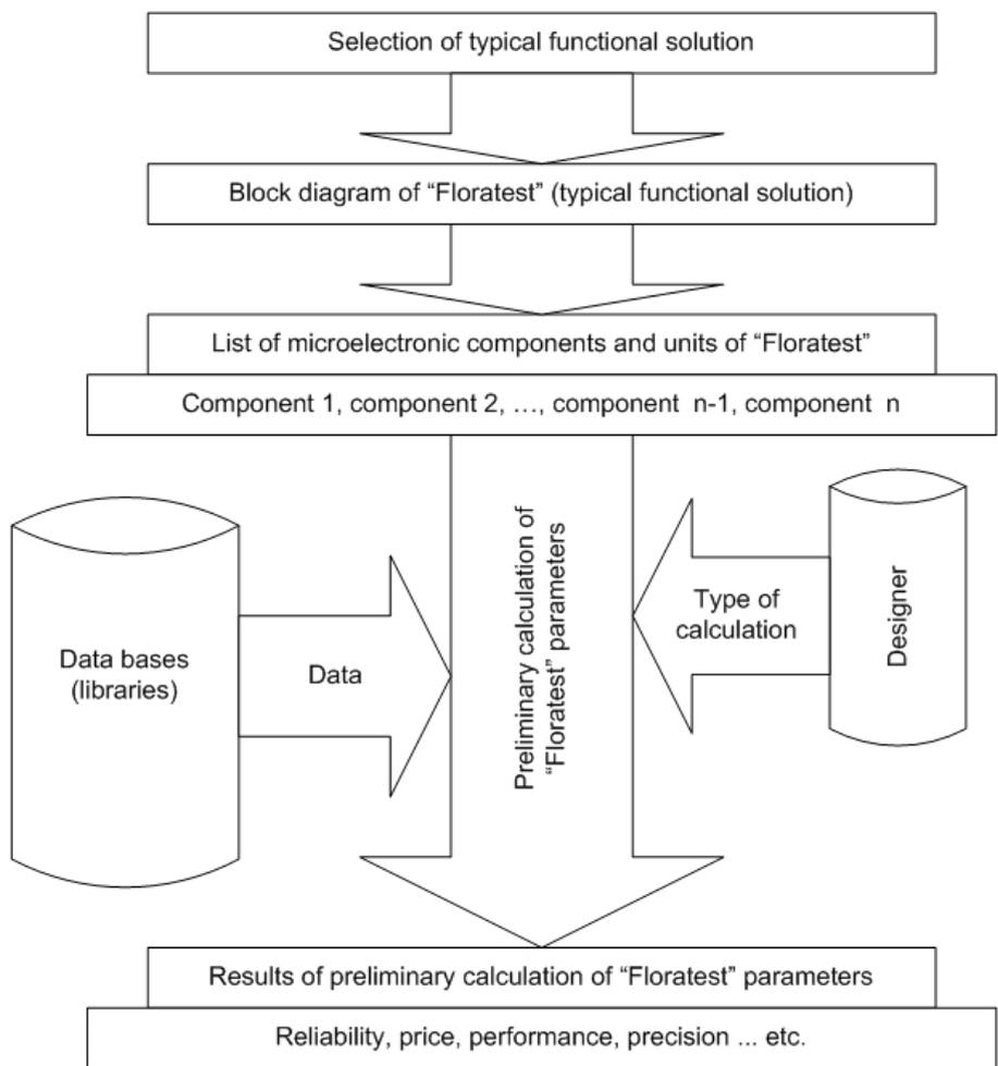
Fig. 7. Designing of "Floratest" by means of virtual laboratory
