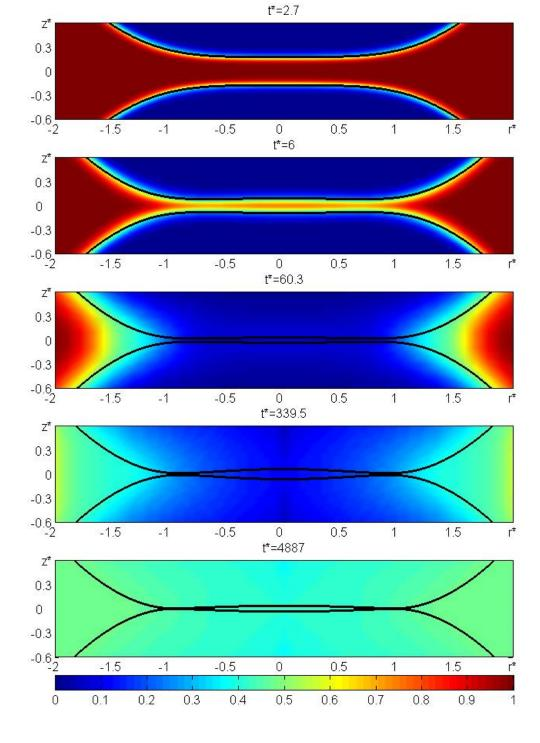
The evolution of the film thickness, h at  $\lambda = 1$ ;  $Pe_s = 10^5$ ;  $Pe = Pe_d = 10^3$ ;  $K = K_d = 0.2$ , case  $C \to D$
