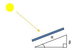
$$\begin{array}{c} \gamma \\ \text{side } \alpha\text{=}0.993m \\ \text{angle} \quad \alpha^{\wedge}\gamma\text{=}\ 28^{\circ} \end{array}$$
