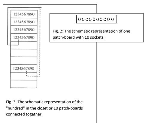
Each pair of wires has a particular place in the patch board (see Fig. 2), so each patch board has 10 places ordered from left to right and from the top to the bottom (see Fig. 3) of the frame (incoming or outgoing).
