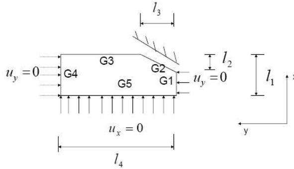
Fig. 1. Scheme of applied on the substratum boundary conditions
