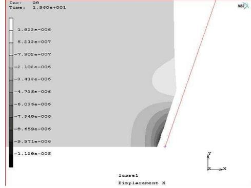
Fig. 4. Field of displacements without applied boundary condition on  $G4$
