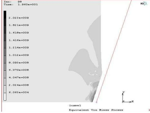
Fig. 3. Field of stresses without applied boundary condition on  $G4$
