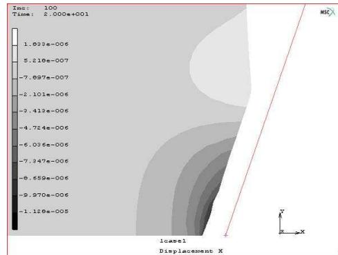
Fig. 6. Field of displacements with applied boundary condition on  $G4$
