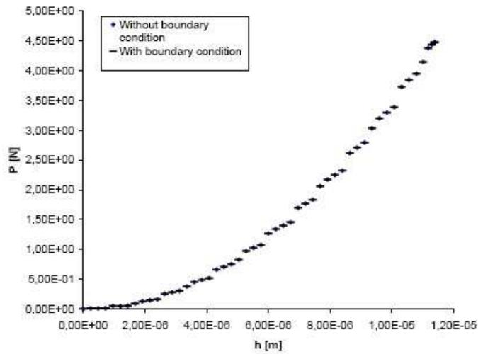
Fig. 2. Load-displacement curve with and without applied boundary condition on G4
