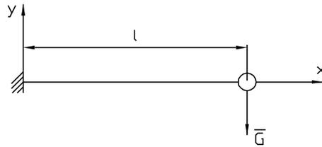
Fig. 1. Cantilever with a fixed point mass at its end
