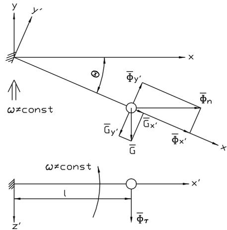
Fig. 5. Rotation of an elastic link in horizontal plane with variable velocity
