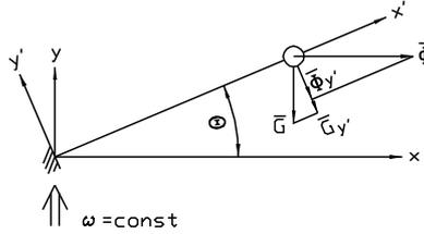
Fig. 4. Rotation of an elastic link in horizontal plane with constant velocity
