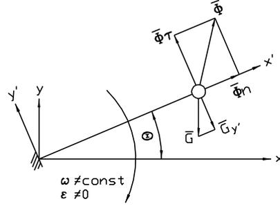
Fig. 3. Rotation of an elastic link in vertical plane with variable velocity
