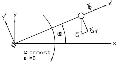
Fig. 2. Rotation of a flexible link in vertical plane with constant velocity
