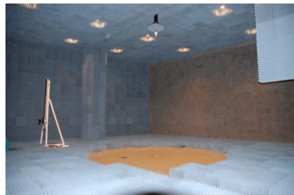
Fig.5 Anechoic Chamber A-METLAB and Plane-Polar Type Near Field Scanner in Kyoto University
