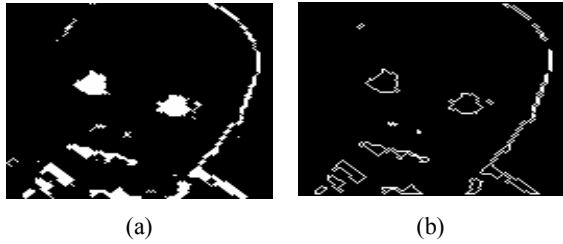
Figure 12: Baby image: (a) Binary image from details coefficients, and (b) Contours extraction using SSPCE method.
