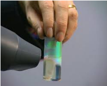
Figure : Dependence of liquid crystal materials on temperature.
