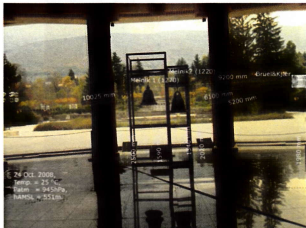
Fig. 2 Measuring microphone toward bell 'Melnik2' disposition.
