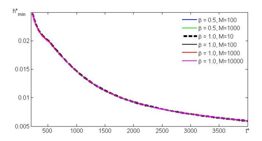
Numerical test: Time discretization. The evolution of the minimal film thickness for different time stepping methods - zoom.
