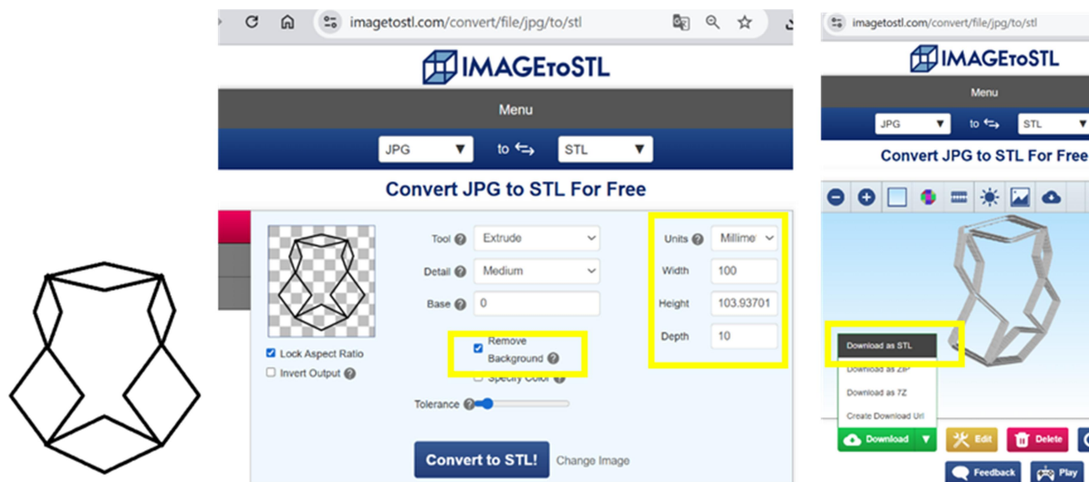
Fig. 2. Generating a 3D model of a jewel from a digitally made file with the background removed
