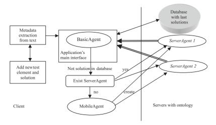
Fig. 1. Scheme of the proposed realization of the system for e-learning tests evaluation
